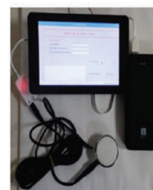
Fig. Developed prototype presenting its components: a low-cost DSP processor with a touch-screen, rechargeable battery, sound card and a stethoscope.
