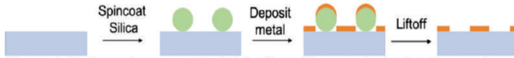
Figure 1: Various steps used for fabrication of the nanohole structures using shadow sphere lithography
