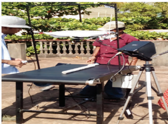
NISA Hyperspectral Core Logger (To be patented) logging drill core samples for Uranium exploration
