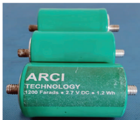
Indigenous developed 1200F Supercapacitor using activated carbon derived from petroleum coke waste
