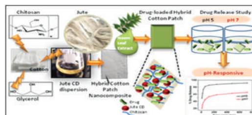
Hybrid cotton patch nanocomposite incorporated with jute carbon dots fabricated for the drug release
