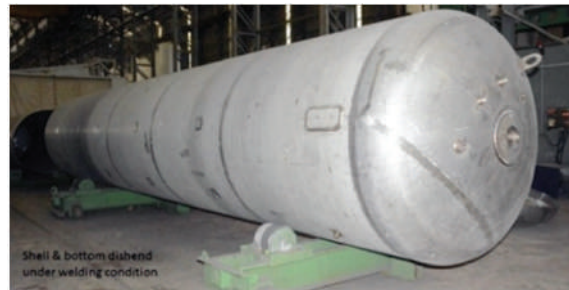
Fig. Cryogenic Tank for liquid argon storage under fabrication (INOX, Vadodara)
