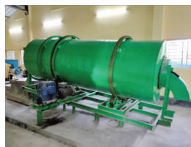
Fig. Image of the continuous rotary drum composter(RDC) installed at IIT Guwahati
