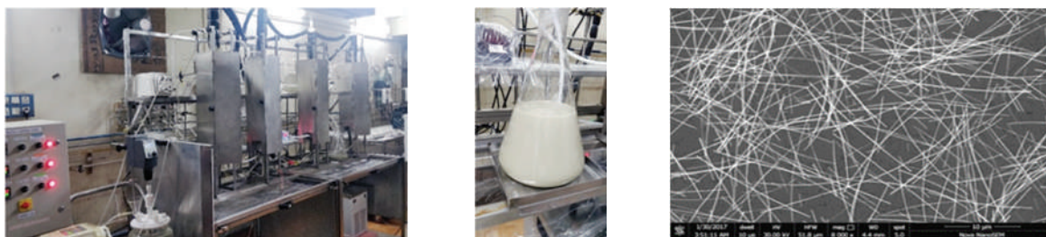
Fig. A continuous process for silver nanowires: (Left) Pilot plant inaugurated on Jan 31, 2020; (Middle) Ag NW suspension collected at the reactor outlet and (Right) FE-SEM image of silver nanowires synthesized in the pilot plant.
