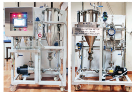
Fig. CSIR-NCL Cavitation Pilot Plant for Wastewater Treatment
