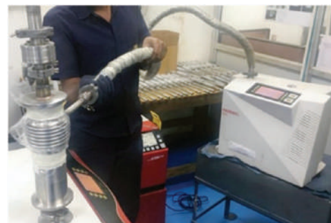
Fig. Fabrication of metal bellow expansion joints in progress (Metallic Bellows, Chennai) Prototype Metal bellows (Left), Leak test of metal bellow expansion joint in progress (Right)
