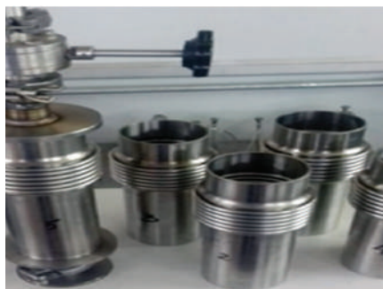
Fig. Fabrication of metal bellow expansion joints in progress (Metallic Bellows, Chennai) Prototype Metal bellows (Left), Leak test of metal bellow expansion joint in progress (Right)
